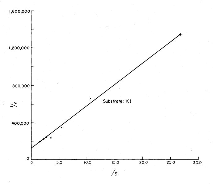
Catalytic Oxidation of Iodide by Air; Plot of Reciprocal Velocity, v, (Moles per Liter per minute) against Reciprocal Sulfuric Acid Concentration, S, (equivalents per liter). Calculated from data of Fig. 24. K<sub>s</sub> = 0.430 V = 1.7 x 10 moles of IO per minute (maximum velocity).
